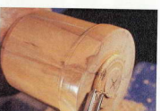
18 Slice off the dovetail with the box held in a jam chuck.
