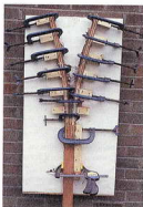
The laminate glued and cramped.
