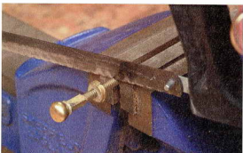
To cut a bolt to length, fit the handle and mark on the length. Remove and screw the nut back onto the bolt before placing in a vice. After sawing to length, file the ragged edge and remove the nut to recut the thread.
