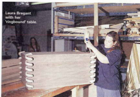
One of two large press presses in the shop, where laminated timber is formed into shapes.
