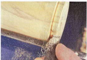
10 Set the tool rest at centre height, then push the chaser across to start the thread.
