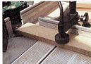
22 Use a biscuit cutter in the router table to slot the ends.
