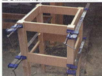
26 Complete the frame assembly ensuring that the radiused edges on the rails are at the bottom.
