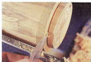
9 Cut a gap at the end of the thread section using a narrow parting tool.
