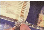
11 Let the threads pull the chaser across once the threads are established.
