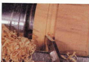
14 Form the moulding at the base of the box with the parting tool.
