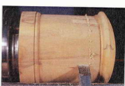
15 Smooth out the sides with the beading tool using the corner of the blade.
