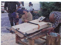
Some sculptors sliced and re-glued their blocks. Gap filling polyurethane glues make it possible to get good bonds, with acceptable glue-lines, in far-from-perfect conditions.
