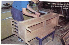
Join the front frame together before assembling to the side frames.
