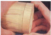
12 Ensure the threads have been cut to full depth before trying on the lid.
