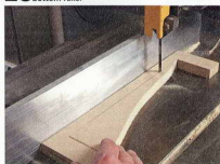
25 Cut the drawer aperture out of one of the bottom rails.
