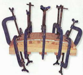
The plywood sandwich cramped to the former.
