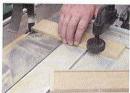
5 A sliding table makes short work of the drawer half lap joint.
