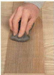
Fine steel wool can break up during use giving a grey tone to open textured woods that haven't been fully sealed.
