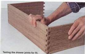
Testing the drawer joints for fit.
