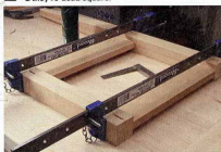
26 Complete the frame assembly ensuring that the radiused edges on the rails are at the bottom.
