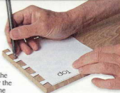
To form the through dovetail joints, make a template for the tails using some thin card.
