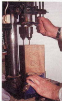
Boring holes for the brass rods.
