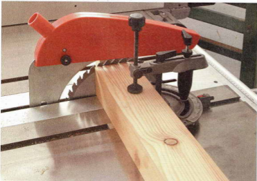
The mitre guide with timber locked in position.
