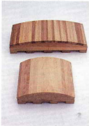
Typical formers used for laminating and bending.
