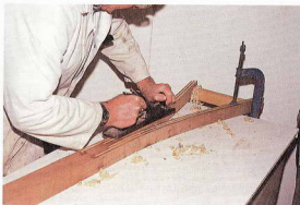
Initial levelling of surfaces using a jack plane.
