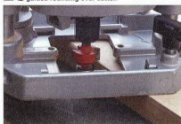
25 Cut the drawer aperture out of one of the bottom rails.
