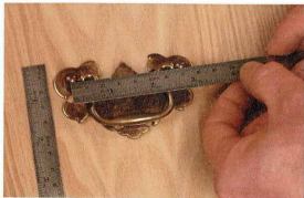
Suppliers usually require several measurements to ensure that the sizes are correct. The height of the back plate and distance between centres are typical.
