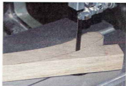
Remove the leg from the lathe then cut off the waste on the bandsaw.
